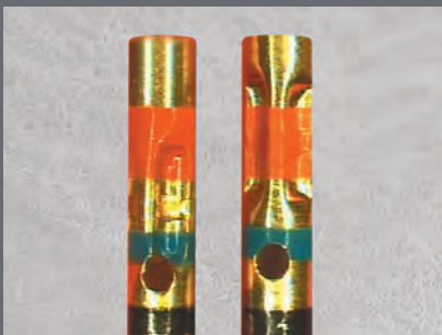
Example of an incorrect crimp on left showing deformation of the inspection hole against a correct crimp on right. Incorrect crimp is caused by incorrect tool settings.
