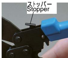
With stopper, useful when store. Depress the stopper while squeezing the handles tightly to prevent the handles expand after use. Do not depress the stopper prior to squeezing the handles. Squeezing the handles gently makes them free.
