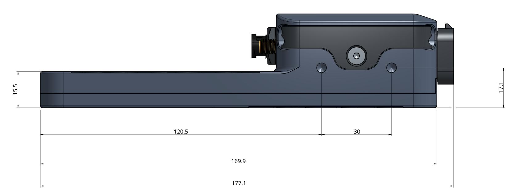
NOTE: SIDE MOUNT THREADS ARE M5 X 0.8. AIM FOR 5 mm OF THREAD ENGAGMENT.
