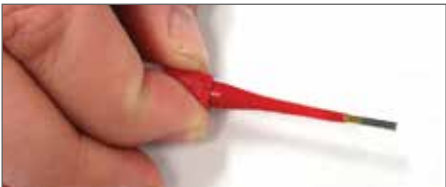
Plastic tool with contact in proper position.
