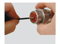
Step 2: Push contact straight into contact cavity until a click is heard/felt. A slight tug will confirm the contact is inserted correctly.
