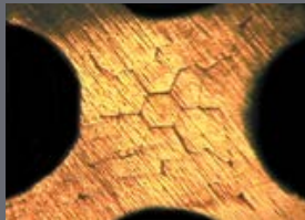
A good crimp showing the individual wires compressed evenly.
